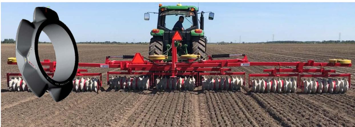
The **TerraStar technology imprints the soil to efficiently create small basins on the surface of tilled soils**. The small depressions increase soil roughness in an orderly fashion which we call Geometrically Ordered Roughness (GOR).
