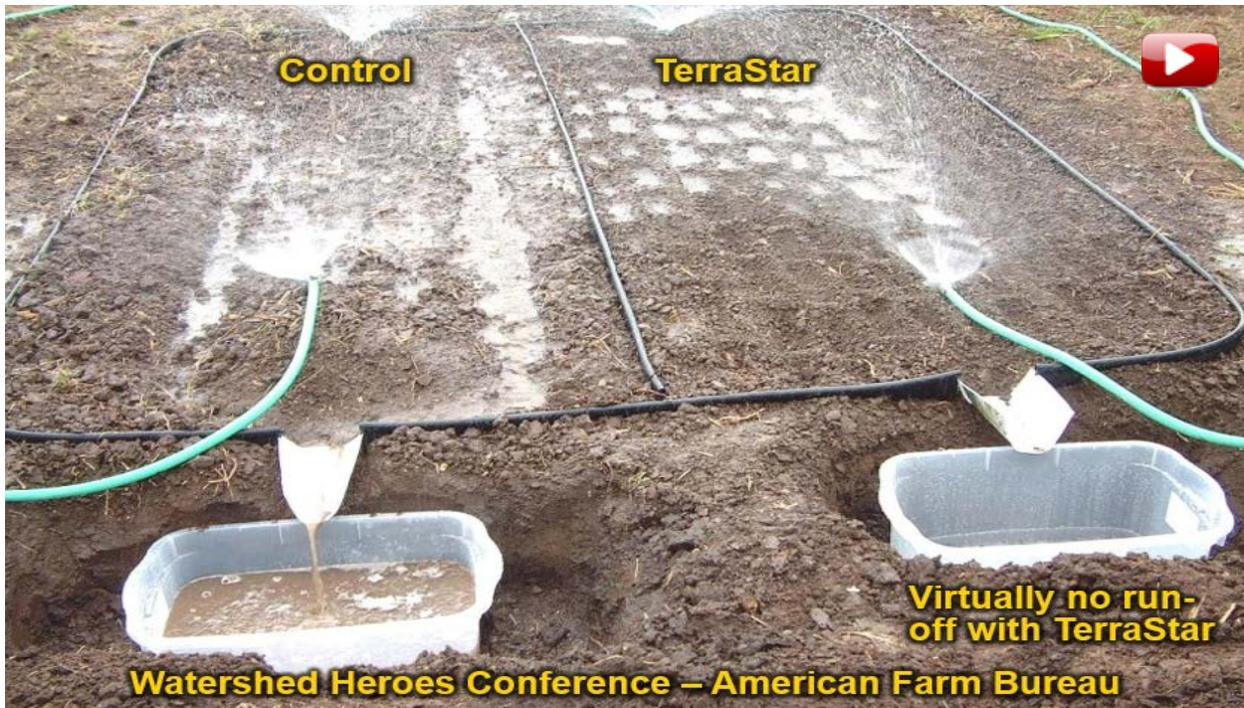
Figure 4. Rainwater detention on a soil surface with GOR
